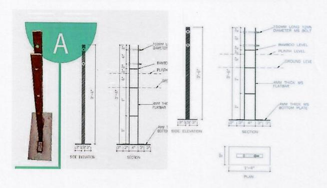
**Steel Footing, Type A** (as per footings catalogue) Width: 38mm, tkn: 4mm, Holes: 14mm dia,
